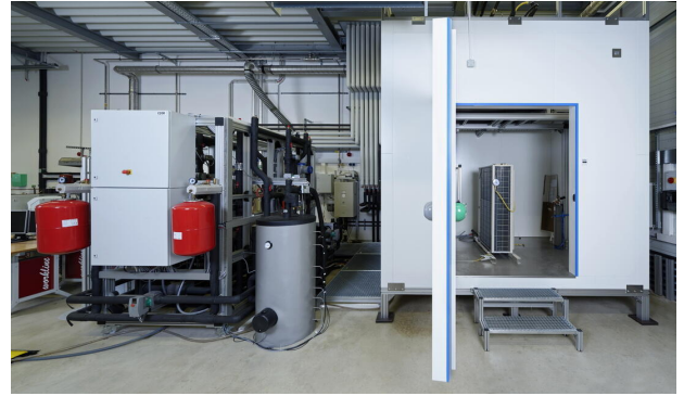
Figure 2: Hardware-in-the-loop (HIL) climatic chamber at RWTH [6].
