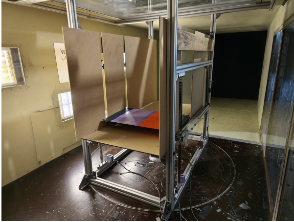
(a) Perspective view of the plunge-pitch dynamic setup (right rear).
