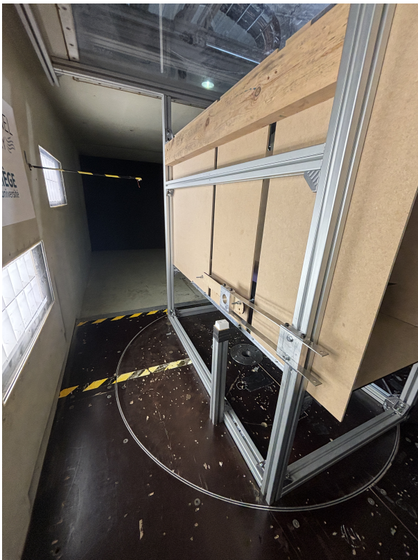
(c) Rear-left perspective view of the plunge-only dynamic setup.
