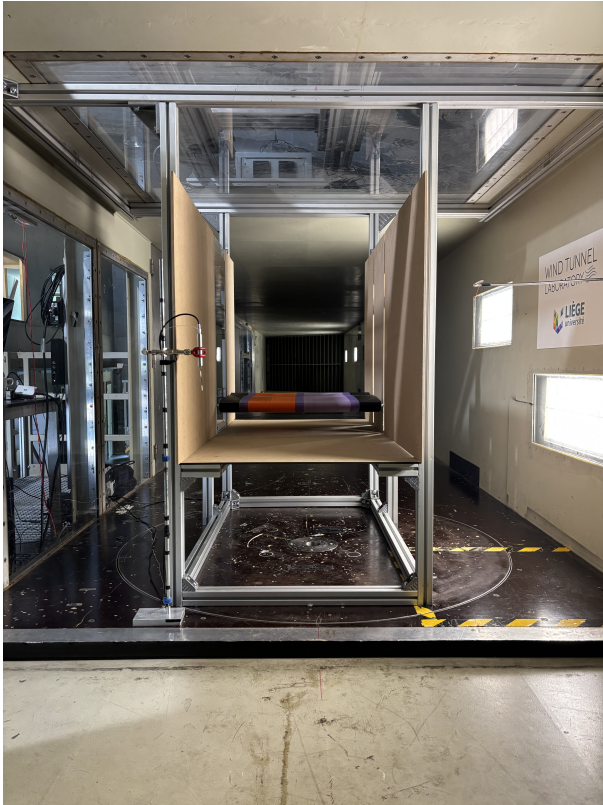
(a) Front view of the plunge-only dynamic setup.
