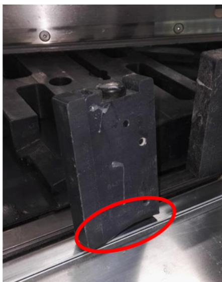
FIGURE 6.10 – Lug de transport principal plié et usé de la Quikflex .
