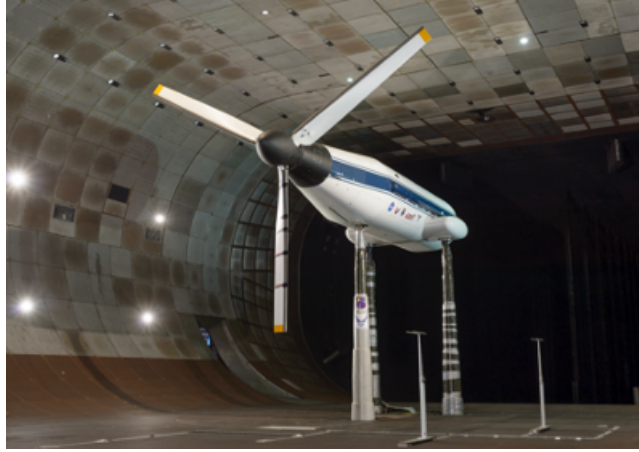
Figure 2.11: NASA tiltrotor test rig (TTR) in the NFAC wind tunnel facilities [30].
