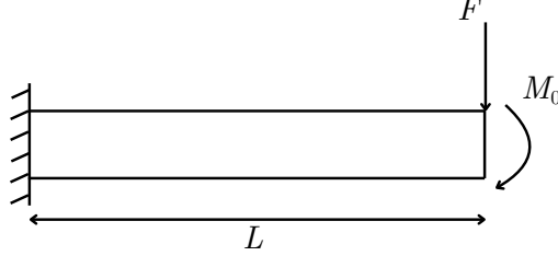
Figure C.1: Cantilever beam of length L loaded at its tip by a concentrated force F and a moment M_0 .
