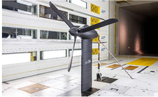
Figure 2.13: ATTILA demonstrator in the German-Dutch wind tunnel large low-speed facility (DNW LLF) 6x6m test section [34].
