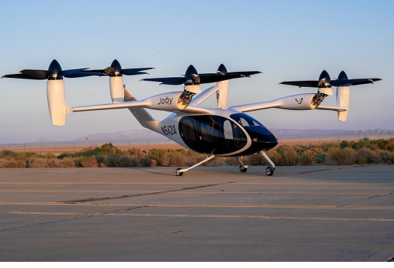
(a) eVTOL Joby Aviation S4, carrying four passengers and one pilot, with six electric motors powering tilting propellers, with a maximum range of 214 km and a maximum speed of 321 km/h [4].
