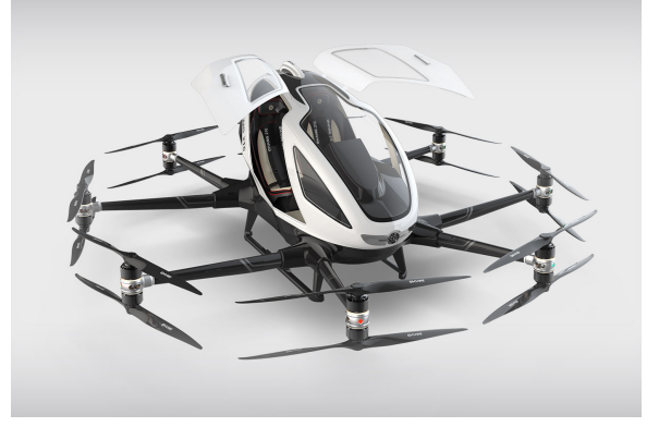
(b) eVTOL EH216, developed by EHang, carrying two passengers, with sixteen independent rotors, with a maximum range of 35 km and a maximum speed of 135 km/h [5].
