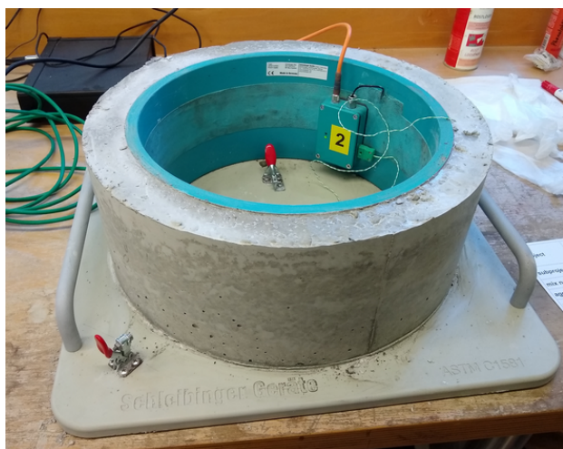
FIGURE 7 – Essai de l'anneau ASTM C1581 (Schleibinger, 2024)
