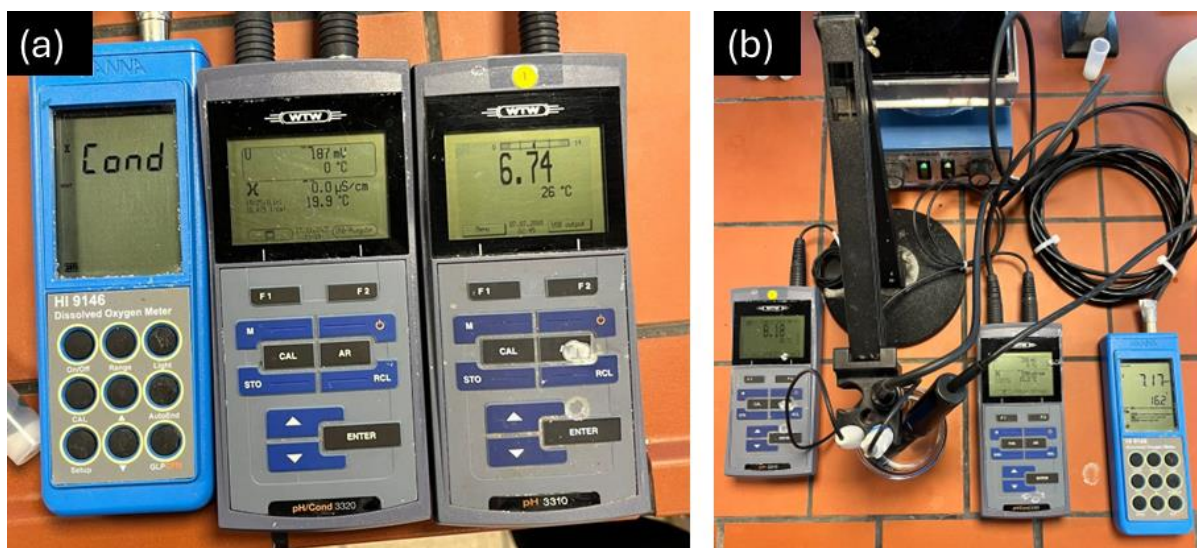
Figure 11. Portable multiparameter probes used for in-situ measurements: (a) handheld devices for pH, conductivity, and DO; (b) complete measurement setup including probes and cables.
