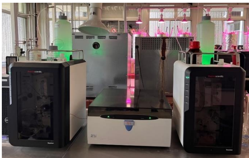
Figure 15. Ion chromatography (IC) systems used for ionic analysis: anion analysis unit (left) and cation analysis unit (right).
