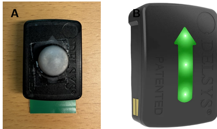
Figure 3.2: Sensors used during data acquisition. (A) IMU combined with a 3D reflective marker attached on top, as used at the three anatomical locations (C7, pelvis, and wrist). (B) Delsys IMU sensor.
