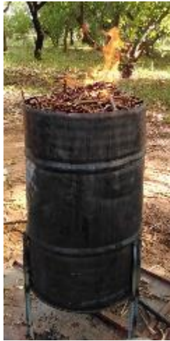
Figure 15 - Top lit updraft oven without chimney
