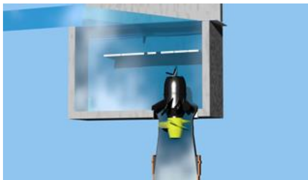
Figure 47: Placement de la turbine Lynx (Turbiwatt, 2009a)
