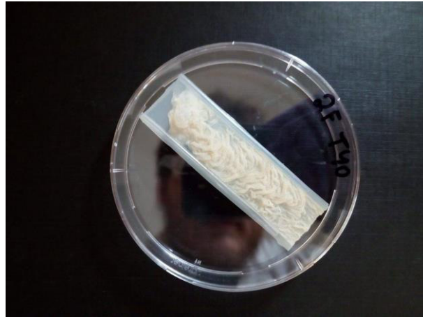
Figure 16: Aspect of a biofilm after 40 hours of continuous cultivation with Drip Flow reactor.
