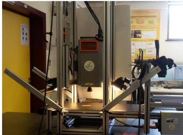
Figure 14: SWIR ImSpector N25E Hyperspectral Imaging System du CRA-W
