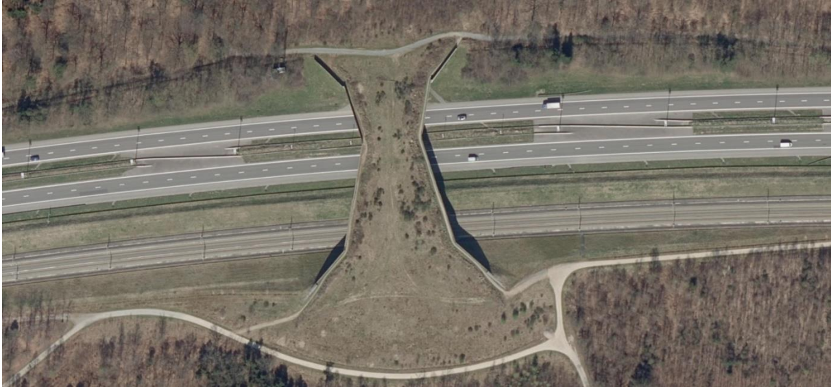
Figure 1 : Overpass for wildlife at Grunhaut, Wallonia, Belgium. Data source : Service Public de Wallonie (SPW), 2015.
