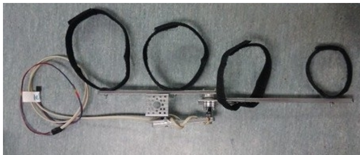
Figure 3.12: Angle sensor - Exoskeleton combined with a potentiometer
