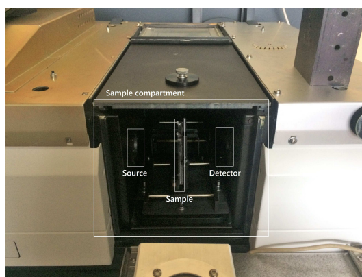
Figure 4.1: Setup of the UV-Vis Cary 6000i spectrophotometer.
