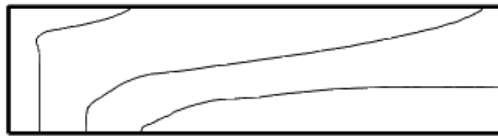
Figure 35: Solid-liquid interface at the midpoint of the mushy region t = 100s, 800s and 1400s . Notice once more that the isothermal lines are parallel to the front, ranging from 212.5K on the solid side to up to 230K on the closest parts of the hot surface
