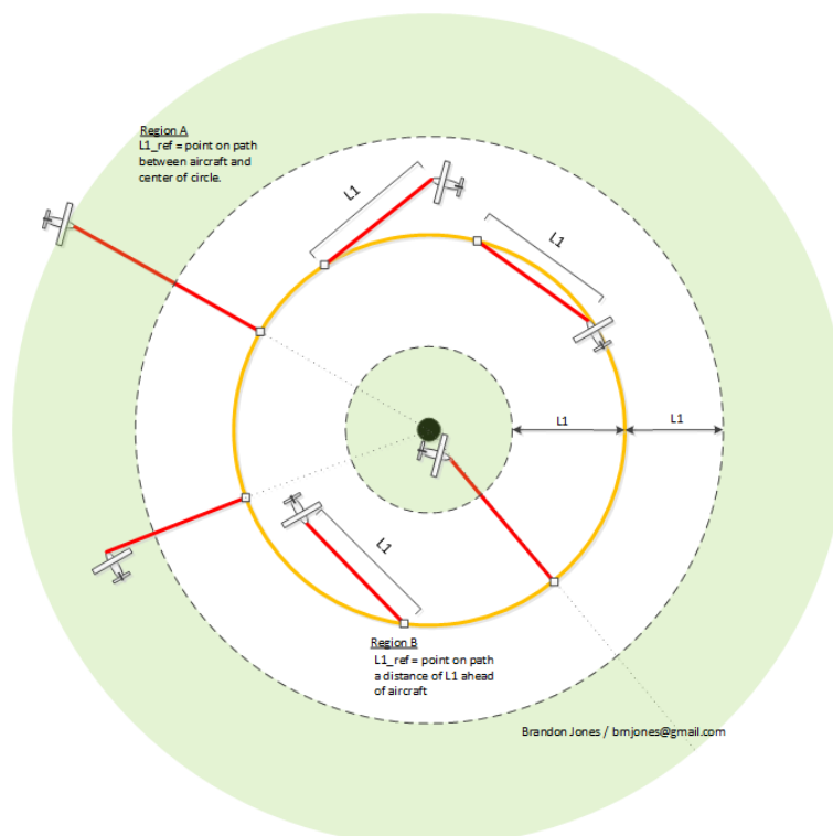
Figure 53: Illustration of the principle of the algorithm for the navigation along a circular trajectory [22].
