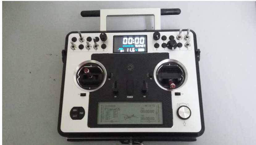
Figure 18: Photo of the radio Taranis X9E .
