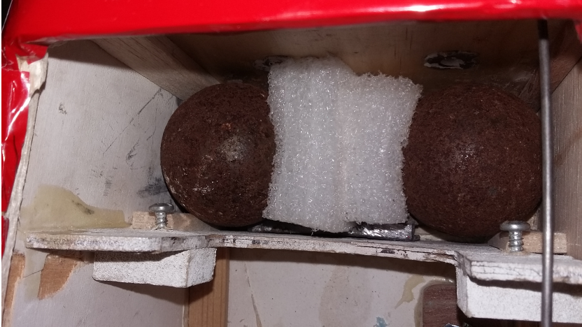
Figure 43: Ballast in the plane. The front of the aircraft is to the top of the photo.
