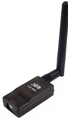
Figure 33: Photo of an antenna used to establish the communication link between the ground station and the plane.
