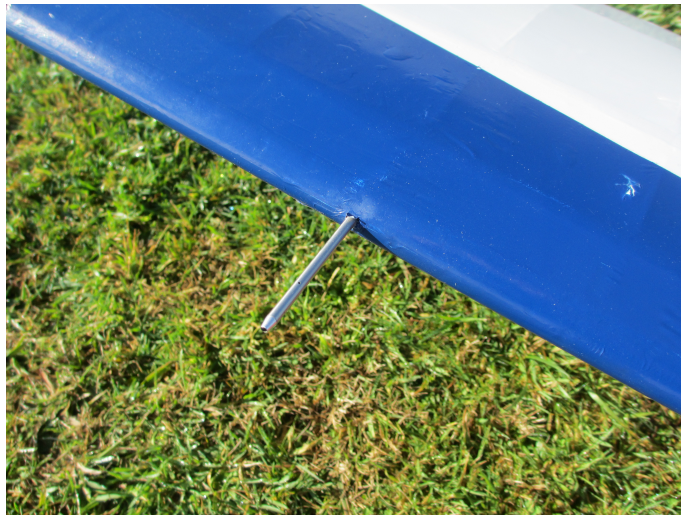
Figure 40: Photo of the Pitot tube installed in the wing.
