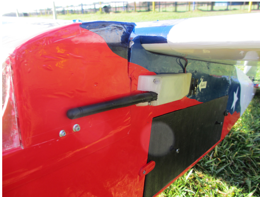
Figure 38: Photo of the antenna mounted on the side of the fuselage.
