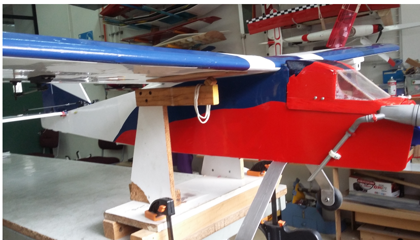
Figure 42: Device used to adjust the position of the centre of gravity.
