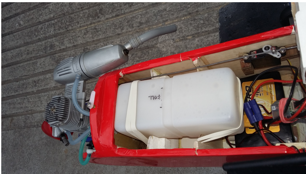
Figure 37: Photo of the battery and the fuel tank.
