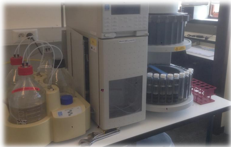
Figure 22: ASE solvent accelerated extractor 200 du LEAE
