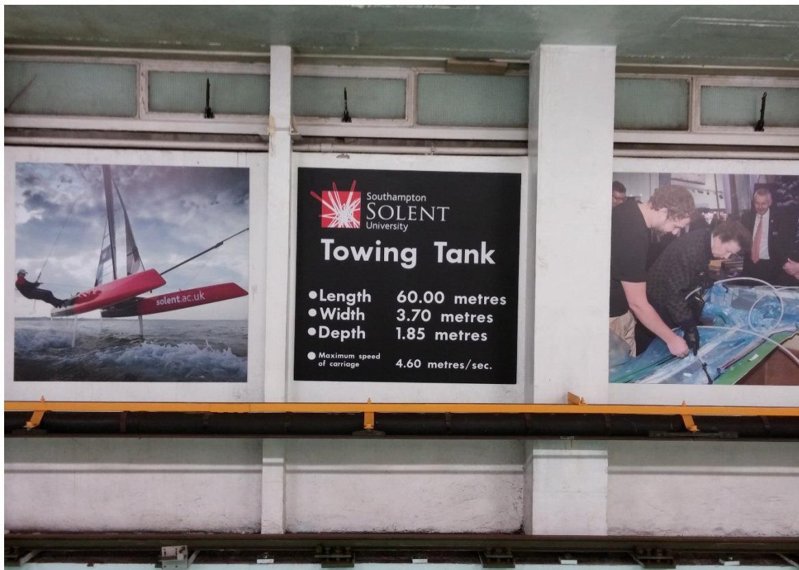
Figure 4-1 : Specifications of the Towing Tank Facility
