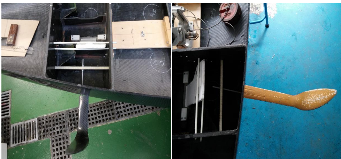
Figure 4-5: Half Curved Dagger Board (Left) & Full Curved Dagger Board (Right)
