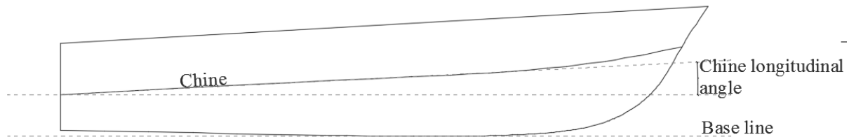
Figure 24. Definition of Chine longitudinal angle.
