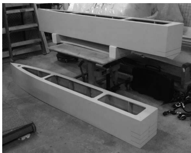
Figure 4. Two types of planning hulls, V and flat bottom. Available from (Clayton, 2013).
