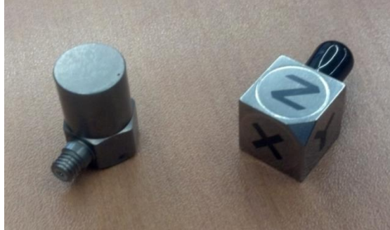
Figure 29- PCB356A02 triaxial at right and PCB3530B unidirectional at left
