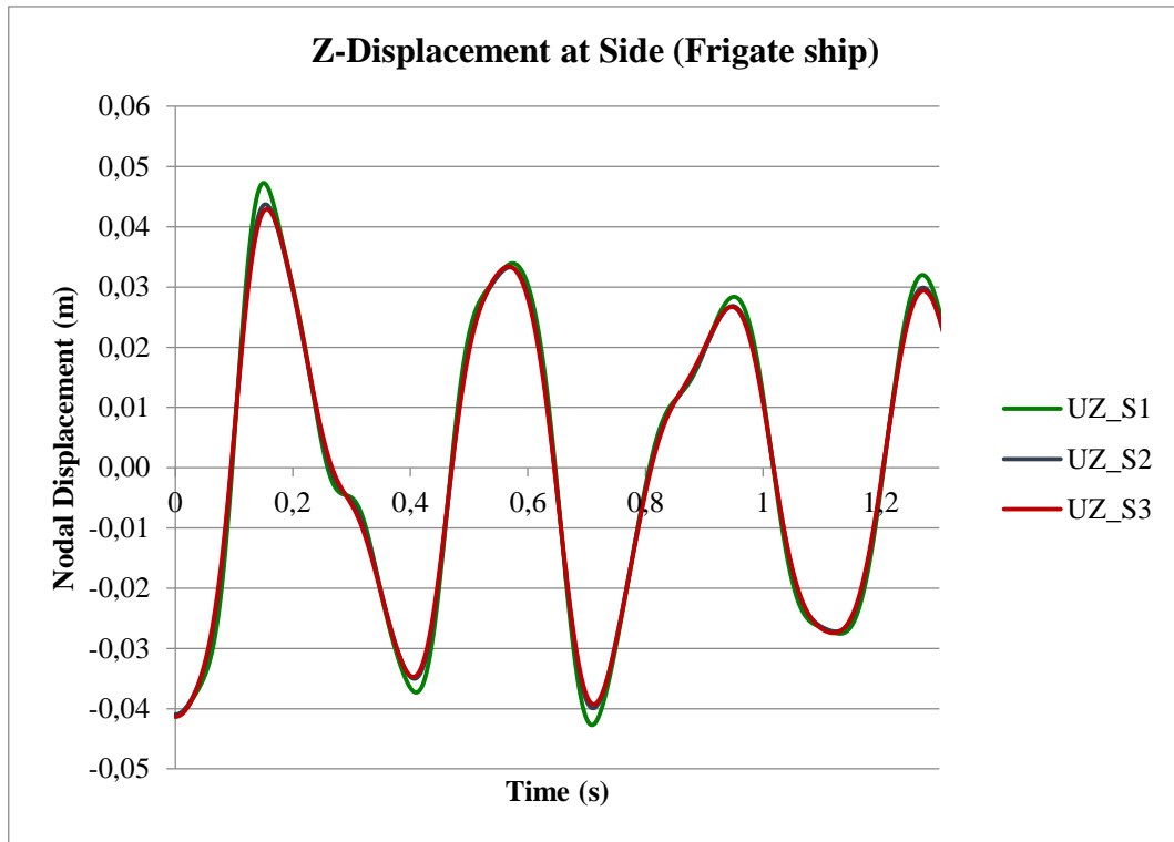
Figure 5.16: Z-displacements at side for frigate ship
