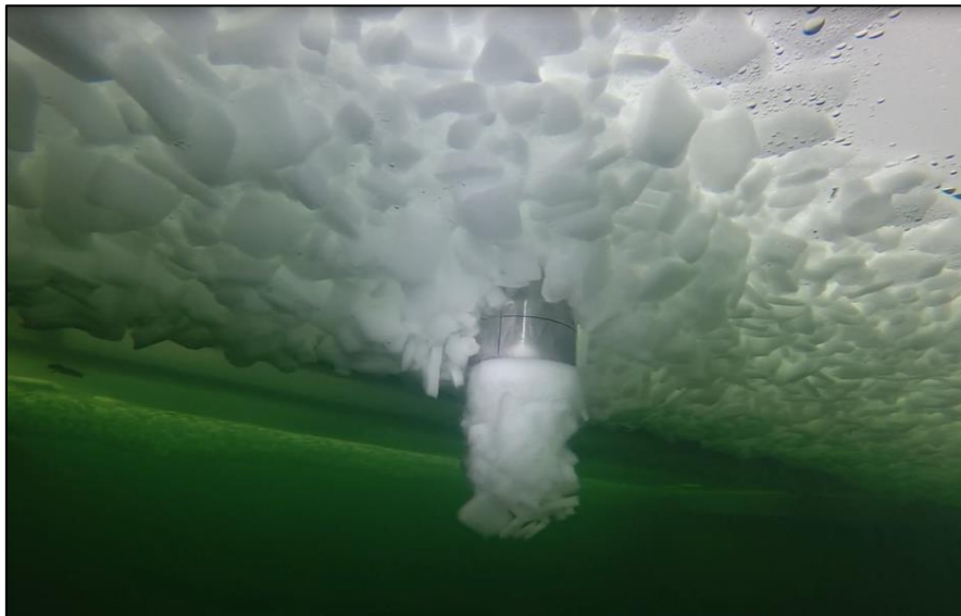
Figure 6. Punch test at HSVA ice basin
