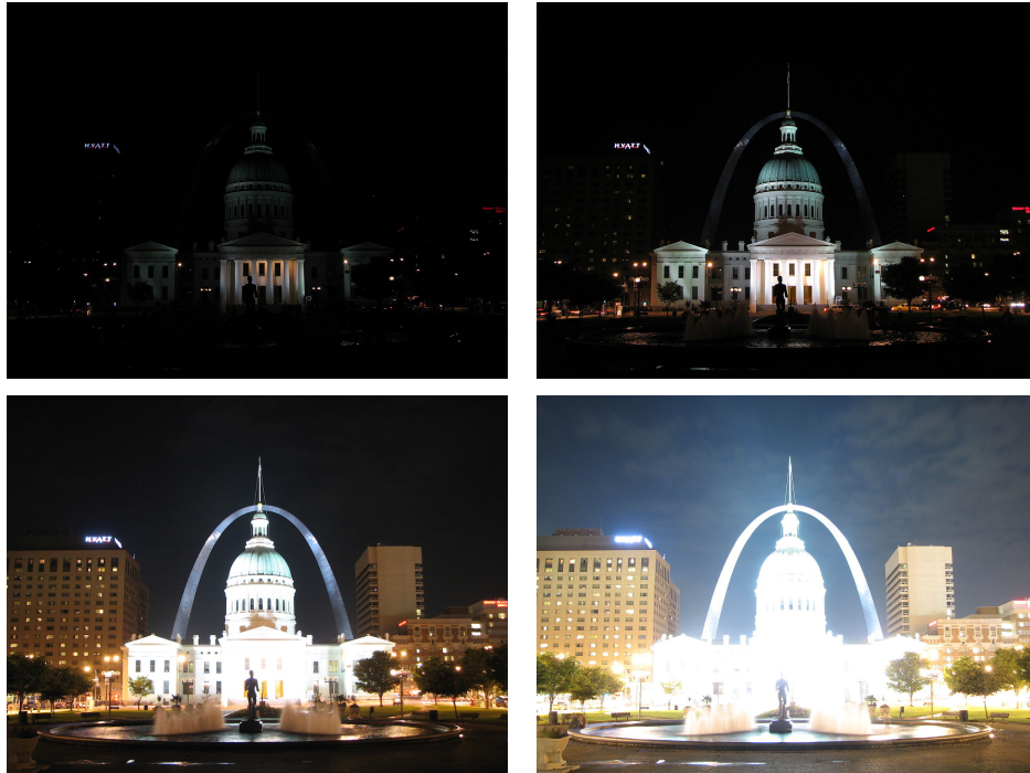
Figure 2.6: Pictures of the same scene taken with an increasing exposure time. The increase between each scene is of +2 stops i.e 4 times longer. Source: wikipedia https://en.wikipedia.org/wiki/High-dynamic-range_imaging
