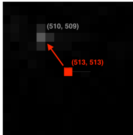
Figure 5.13: Zoom on the output of the phase correlation method applied to contours.
