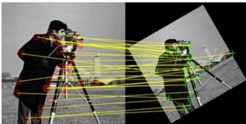
Figure 5.1: Example of feature points in the image used for matching two images. The warping here is a translation, a rotation and scaling. Source: https://nl.mathworks.com/discovery/image-registration.html
