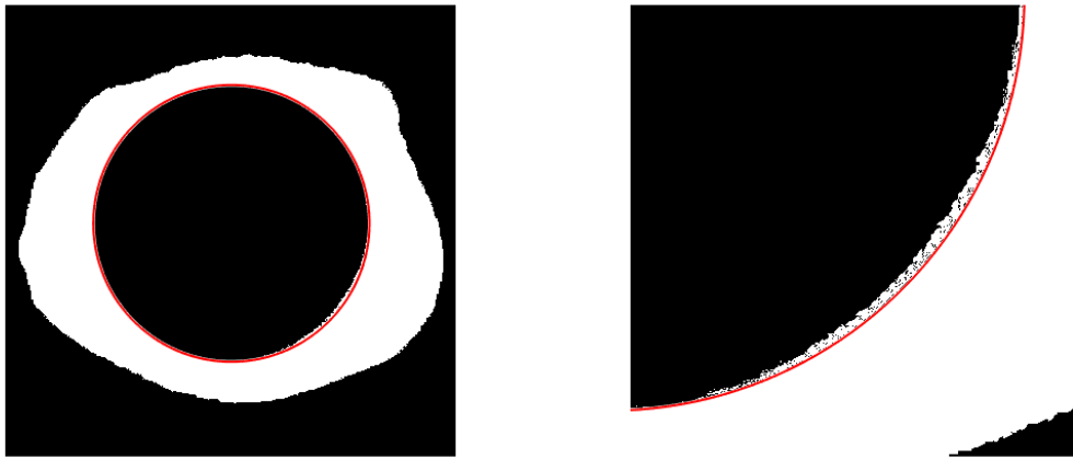
Figure 4.9: Left: binarized image of long exposure. Right: zoom on a part of the circle where glare of light causes the circle to be imperfect
