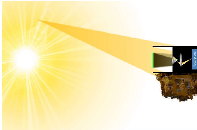
Figure 2.2: Simplistic representation of a coronagraph. The occulter (green) blocks out the direct light from the sun to create an artificial solar eclipse. It allows other parts of the corona to be visible. Copyright ESA–D. Galano
