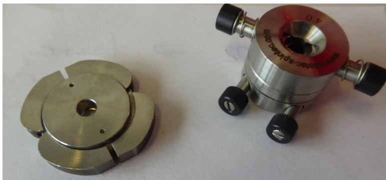
Figure 48: Two types devices, designed for the cap removal of 4 mm rotors
