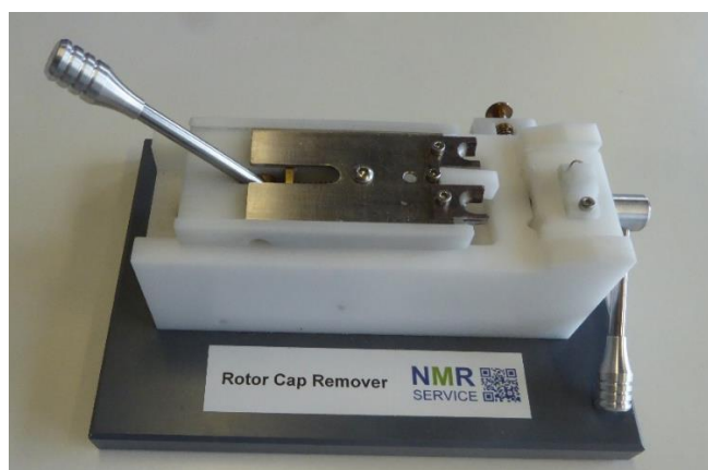
Figure 47: Another device, designed for the cap removal of 4 mm and 2.5 mm rotors
