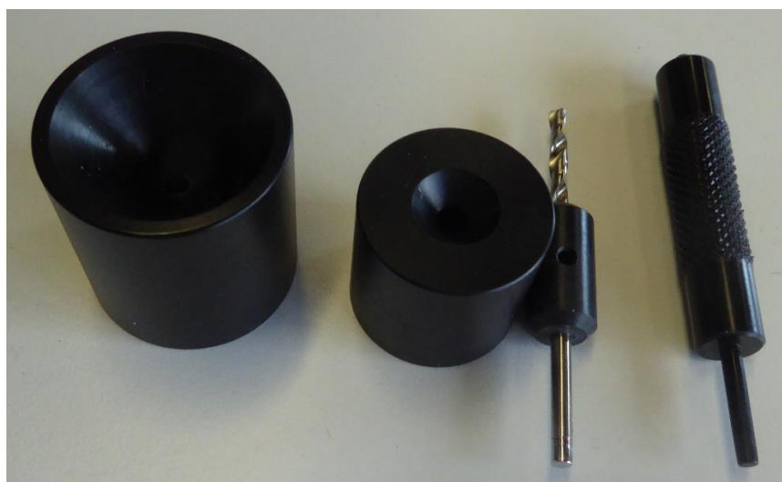
Figure 46: The different filling devices used during this work, adapted to 4 mm rotors and caps
