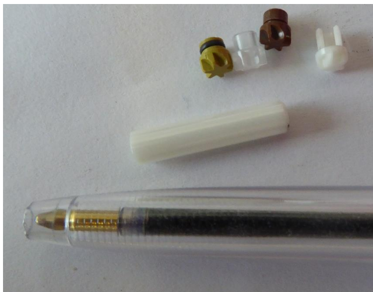
Figure 18. Picture of a 4 mm ZrO 2 rotor and four different kinds of suitable caps, made of Torlon (yellow, with O-Ring), Kel-F polymer (transparent), Vespel (brown, without O-Ring) and ZrO 2 (white, broken). The tip of a ball pen is shown, in order to indicate the small size of the devices.
