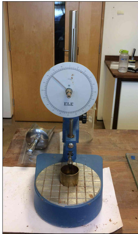
Figure 3.6: Cone penetrometer used to evaluate liquid limit
