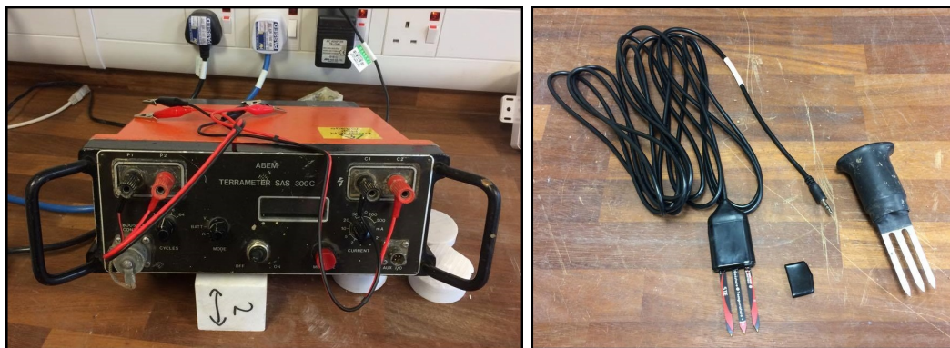
Figure 3.5: ABEM Terrameter SAS 300C (left) and 5TE probe (right)
