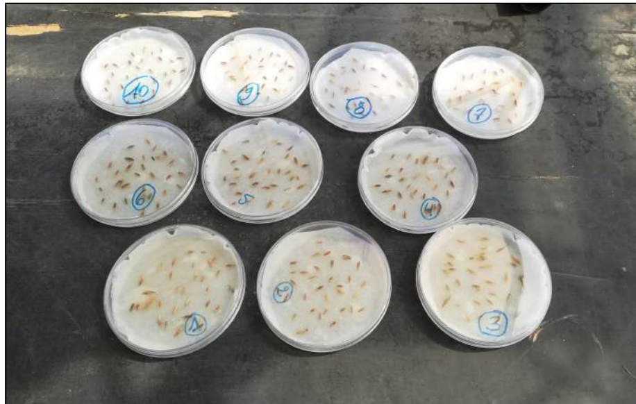
Figure 18: Germination test setup, each 10 cm petri dish contained 30 seeds on humid geotextile, n=10.
