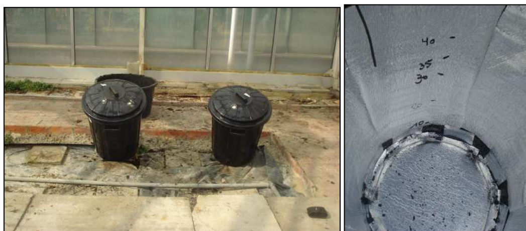
Figure 15: left: set up of the compost bins; right: insulated inside wall of a bin.
