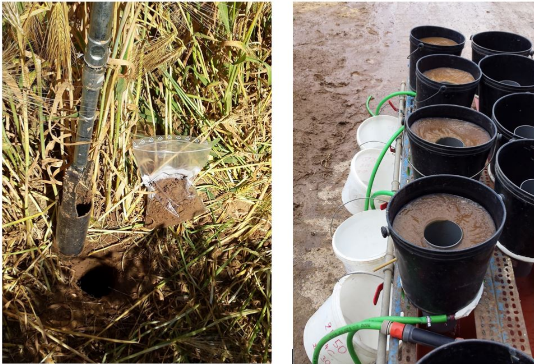
Figure 15: The left picture shows the soil cores that are sampled manually with an auger in the field. The right picture shows the device to separate and wash the roots from the soil samples.
