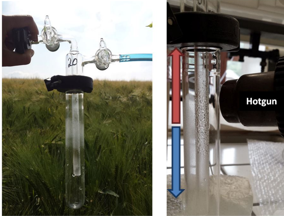
Figure 9: The left picture shows a soil sample water (extracted at 20 cm) in the trap. Condensation can be seen on the rim of the trap. The left picture shows the temperature gradient made with a hotgun (blowing air at 250°C) in the upper part and dry ice in the lower part.
