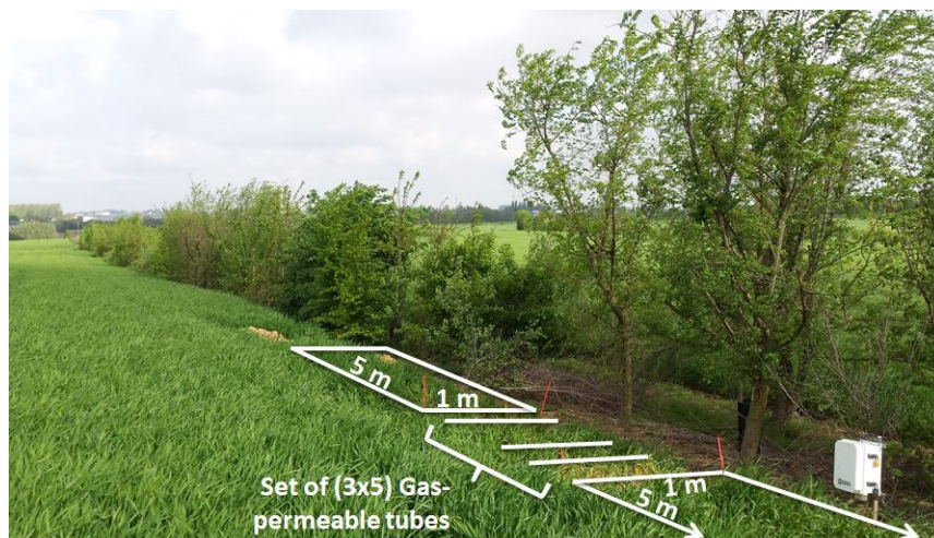
Figure 14: Schematic design of the plant's sampling zone, located in the white frames.
