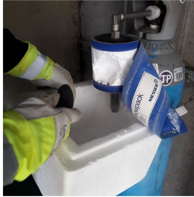
Figure 11: Design and picture of the dry ice making in order to cool the soil water vapour and force condensation of water vapour extracted.
