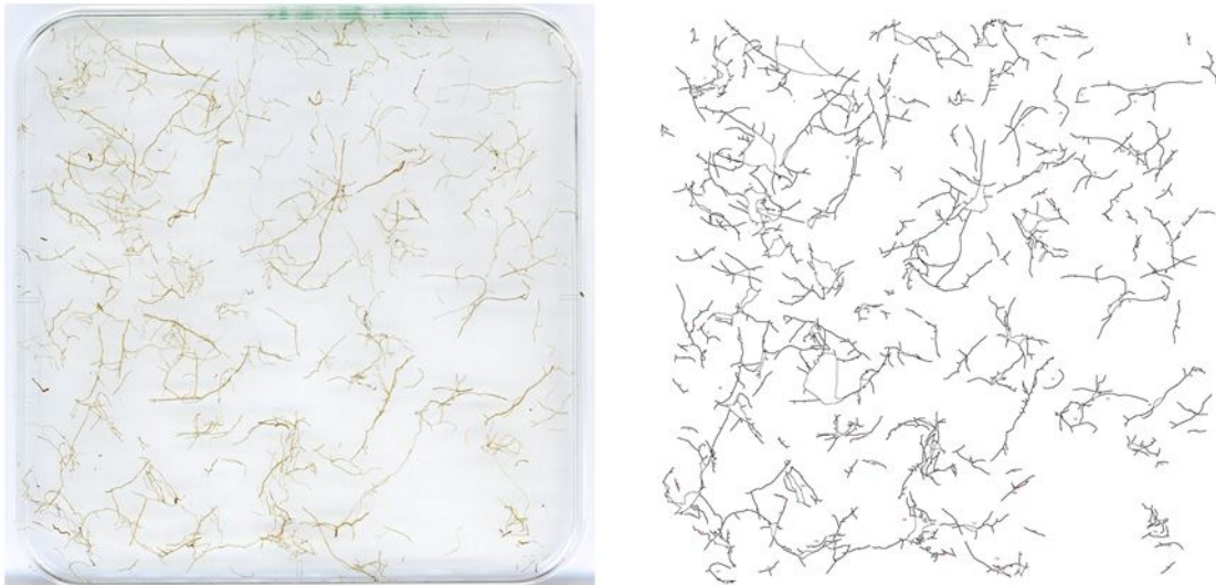
Figure 17: Example of transformed and analysed image with ImageJ; the left picture is a scan of the roots and the right picture is the same image after treatments.
