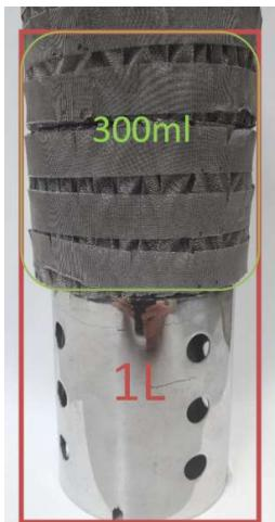
**Figure 26 :** The hollow support with packings. The 1L of medium introduced in column in red and the part in contact with packings (300ml) in green
