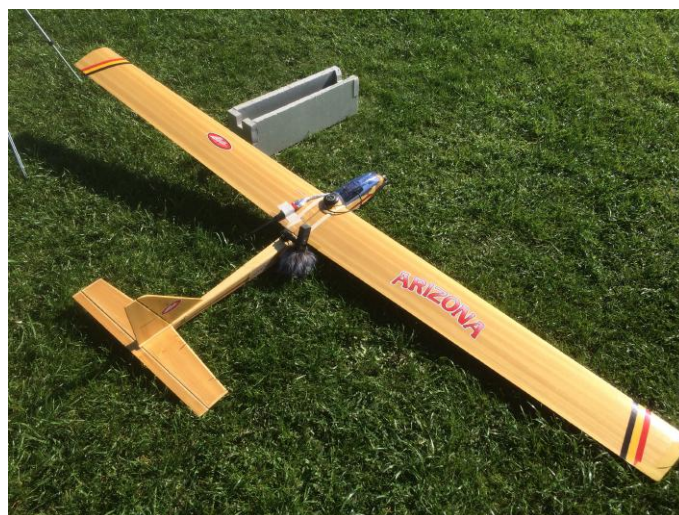
Figure 4. Second fixed-wing drone tested and equipped with the ZOOM H1 Handy Recorder
