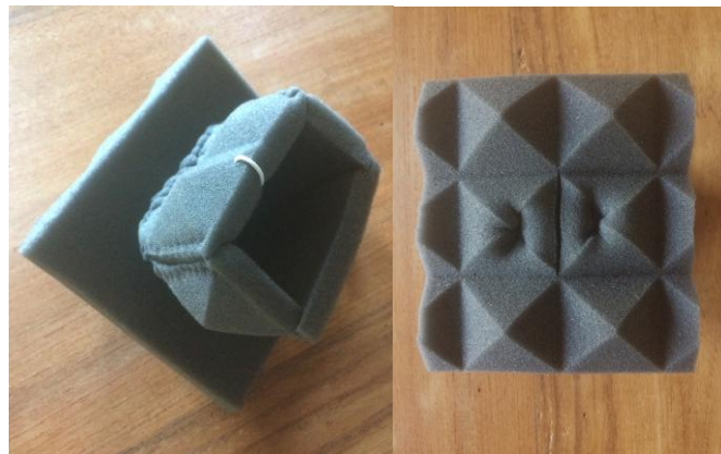
Figure 6. AudioMoth insulation casing with a 26 kg/m 3 density pyramid foam (casing = 6x8x7 cm; top = 13x15 cm)
