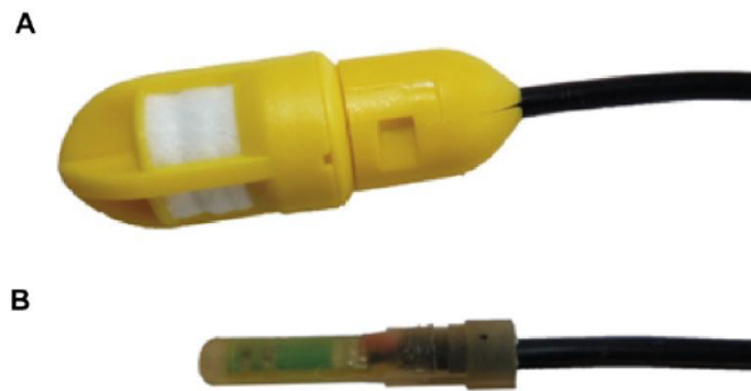
Figure 17: A: PlantCare sensors ; B: sensor without the synthetic felt (Matile et al., 2013).
