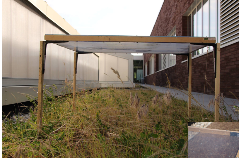
Figure 20: Point-quadrat device for measurement of relative plant coverage (Credits: Julie Reniers).
