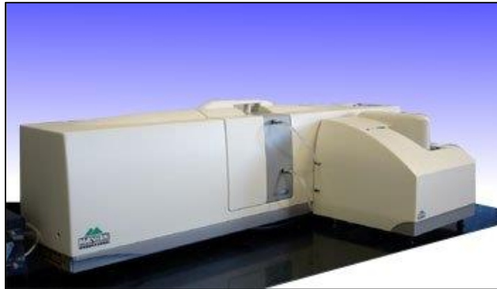
Figure 34: Laser diffraction spectrometer Malvern Mastersizer 2000 [81].
