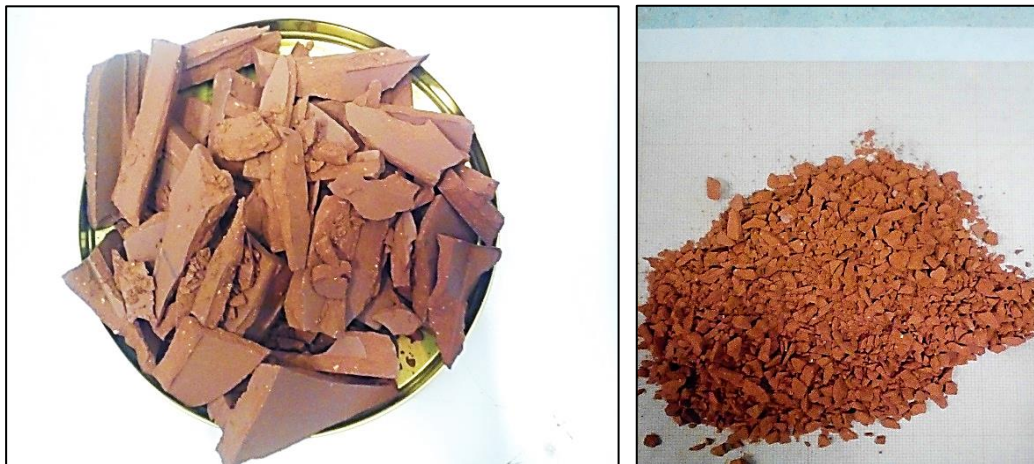
Figure 50: 0/10 mm bricks' fraction, on the left, and brick's sand 0/4 mm, on the right
