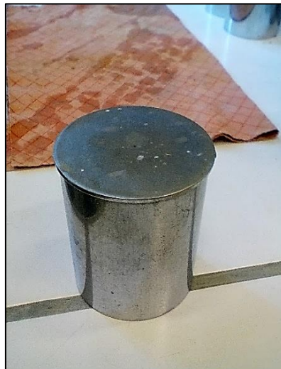
Figure 26: The stainless-steel pycnometer used for the volumetric mass analysis on the brick sand.
