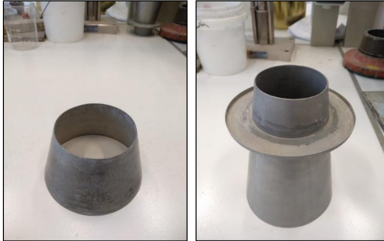
Figure 51: Mini cone (right) and MBE cone (left) for the slump tests.
