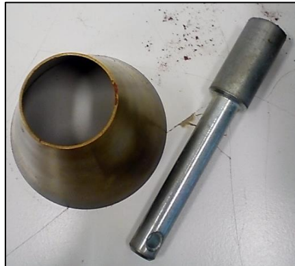
Figure 27: Steel cone and pestle for the NF EN1097-6 test.
