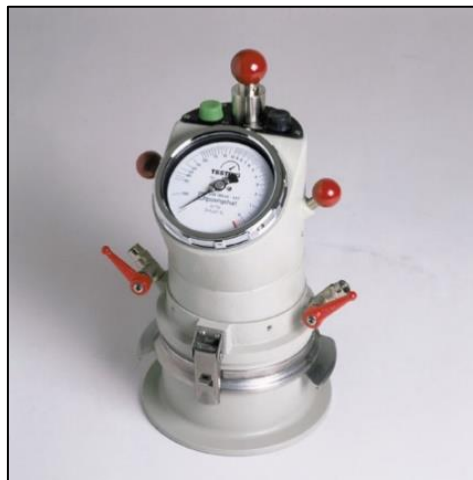
Figure 52: Aerometer of 750 ml for mortar analysis [86].
