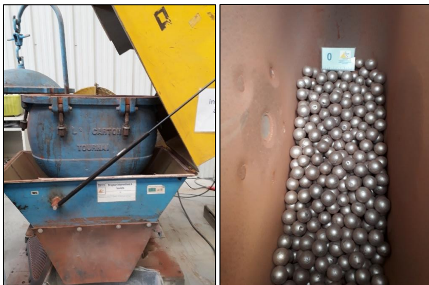
Figure 23: The ball mill outside, on the left, and inside, on the right.
