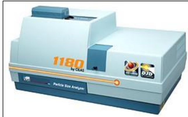
Figure 36: Particles size analyzer CILAS 1180L [83].
