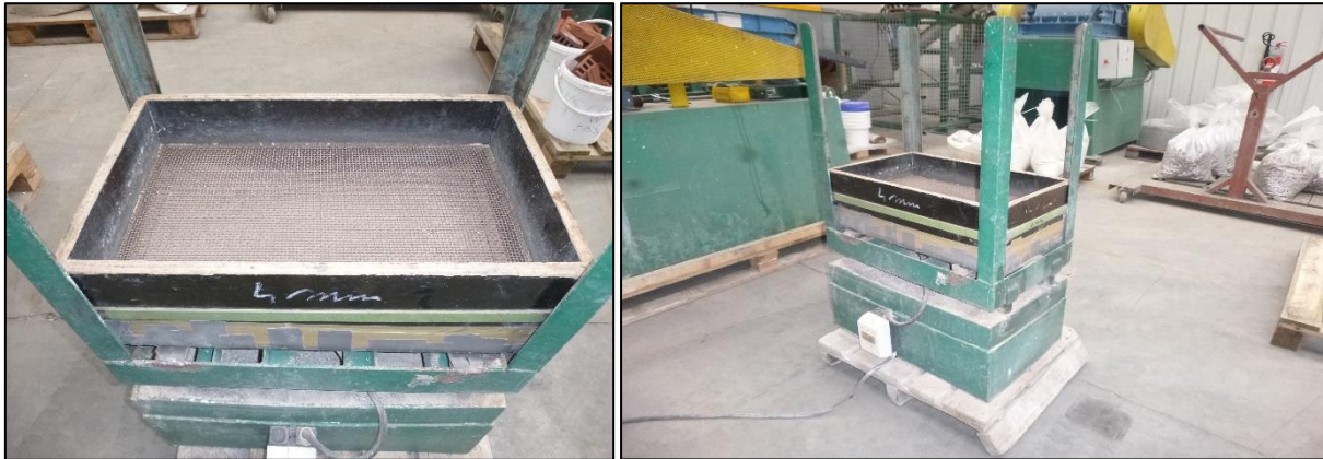
Figure 22: Sieve employed for the separation of the fraction under the 4 mm of dimension.
