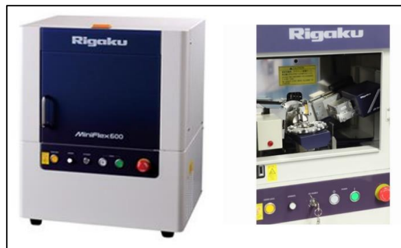
Figure 43: Rigaku MiniFlex 600 for the mineralogical and chemical analysis (Rigaku, 2018).
