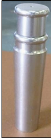
Figure 32: The container used for the Blaine test for the specific surface area [80].
