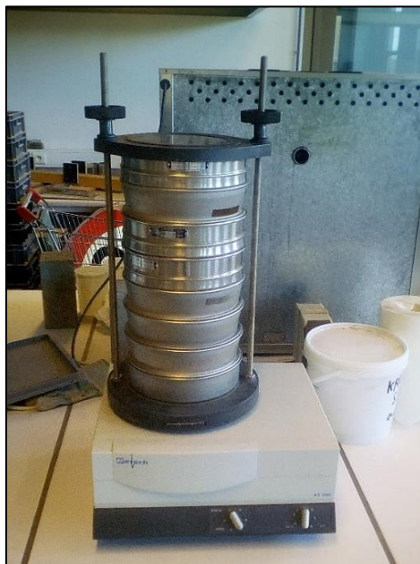
Figure 37: the vibratory sieve shaker AS200 by RETSCH.
