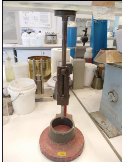
Figure 31: The apparatus for the Vicat test.
