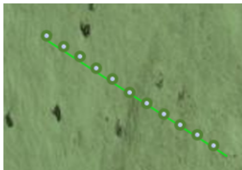
Figure 3.19: Bone B optical picture. The dots are separated by 20\ \mu m . The dots colour represent the quality roughness, here they are green so the roughness is good. The points are close to the line without being on it each time, depending on the SPM analysis results.
