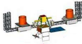
Figure 2.17: The deployment of the SPIRIT, rotation of the first hinge by 90^\circ .
