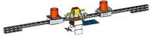
Figure 2.19: The deployment of the SPIRIT, rotation of the third hinge by 180^\circ .
