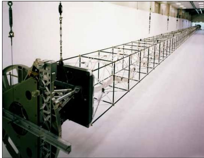
Figure 2.14: The Able Deployable Articulated Mast (ADAM) by NASA [12].
