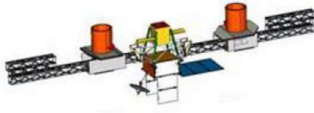
Figure 2.18: The deployment of the SPIRIT, rotation of the second hinge by 90^\circ .
