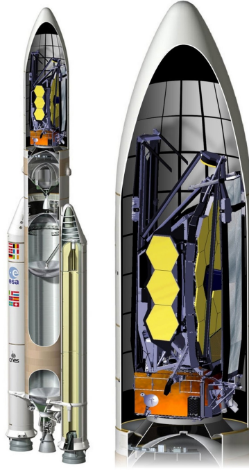
Figure 2.8: The James Webb Space Telescope in the fairing envelope of Ariane 5 [7].
