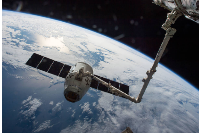
Figure 2.26: The SpaceX Dragon Cargo hold by the Canadarm2 in the ISS [18].
