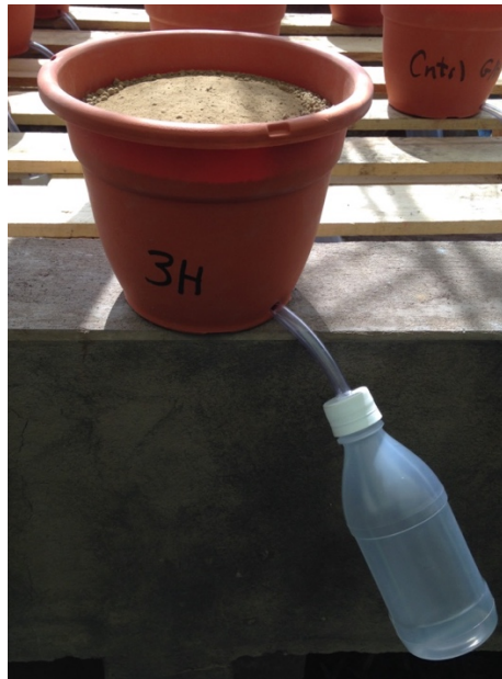
Figure 9: Chemical amendment pots connected to plastic container to collect leachates.
