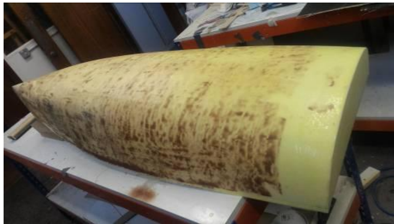
Figure 55: Resin and micro balloons paste covering. Own picture.
