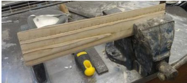
Figure 62: Keel fin plywood laminates. Half of the sanding process. Own picture.
