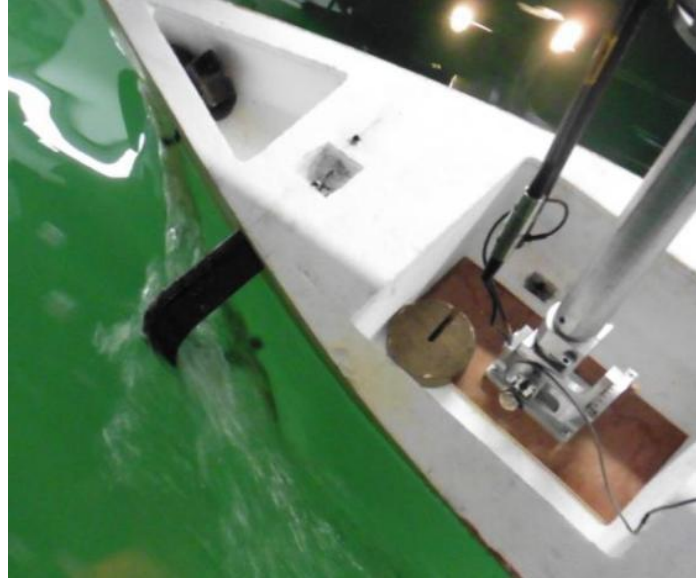
Figure 81: Vortex generation from the bow and interference with Figaro foil at high speeds in the tank. Own picture.
