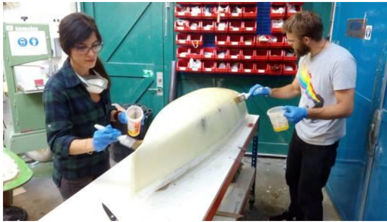
Figure 54: Hand lay-up process in the workshop. Own picture.
