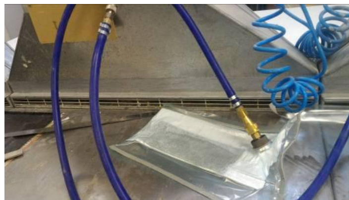
Figure 66: Vacuum bagging process (DSS foil). Own picture.
