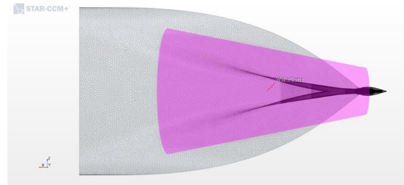
Figure 63- volumetric source for wake field (top view )
