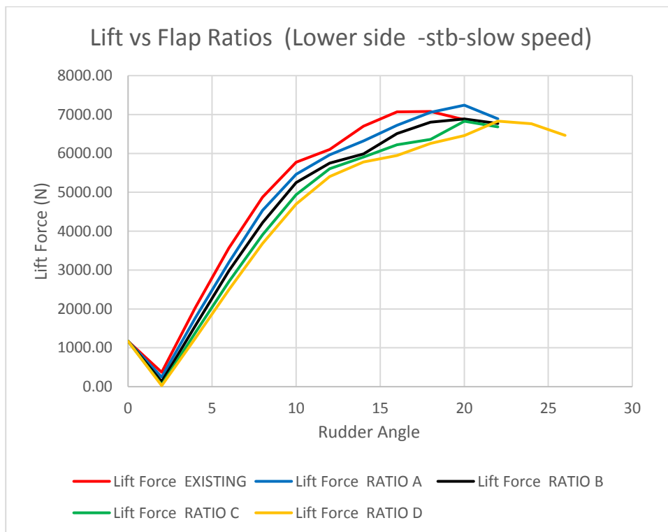
Figure 13-section at lower side -0.7R ,Rudder and flap rotating to stb side at slow speed
