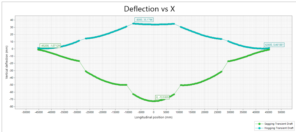
Figure 36: Vertical deflection along the length in sagging and hogging docking condition
