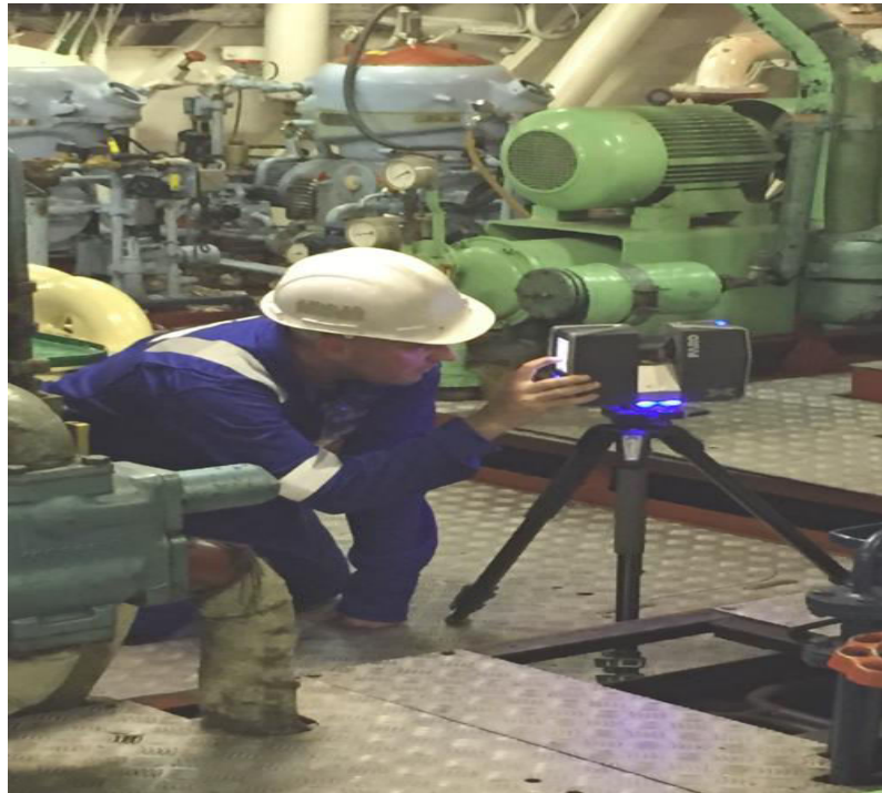
Figure 54: Laser Scanning onboard ship [49]
