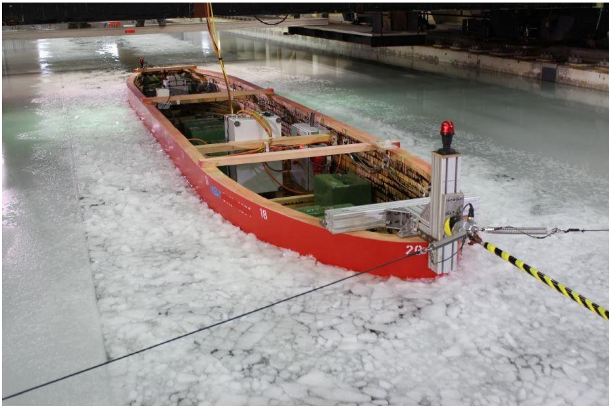
Figure 49: Brash ice model test in ice tank
