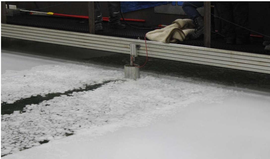
Figure 33: Cylinder experiment in ice tank
