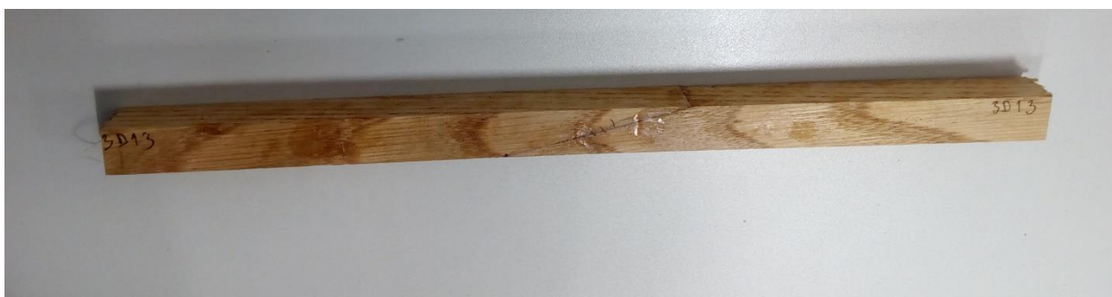
Figure 49– Sample before breaking test
