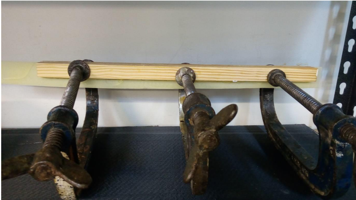
Figure 77 – Sample curing under pressure
