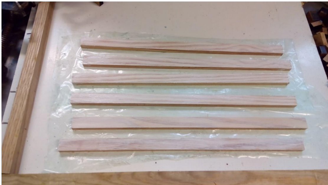
Figure 74– Samples with layer of primer applied
