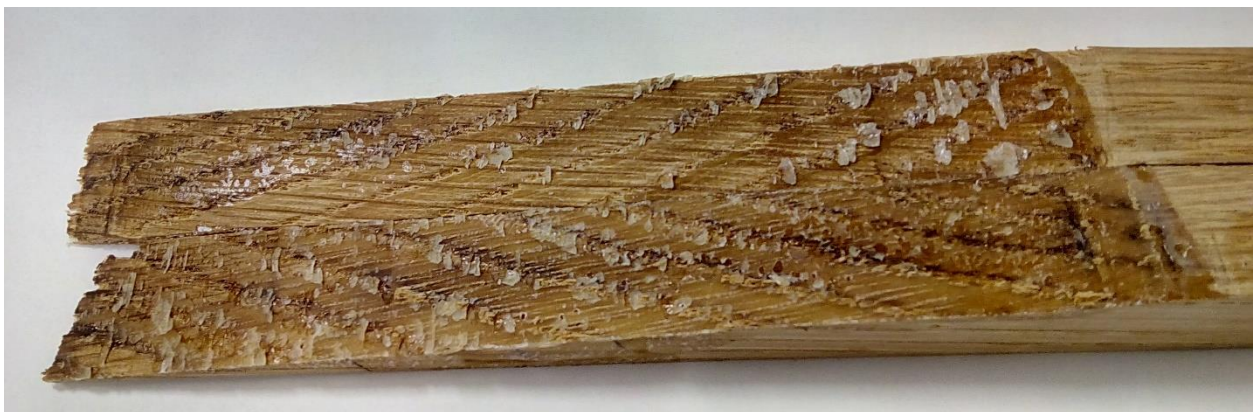
Figure 57- Micro wood failures that match annual ring grains
