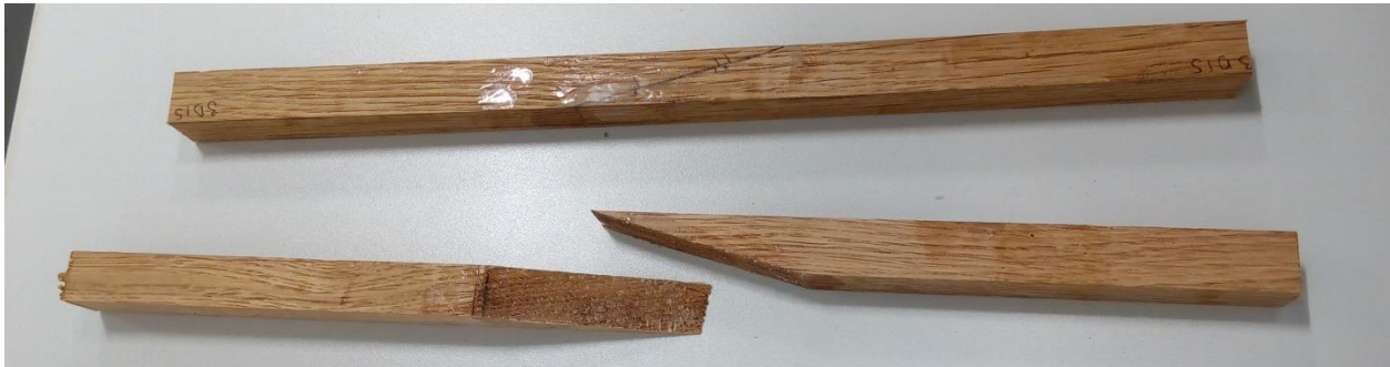
Figure 56 - Samples from 1:4 scarf ratio group
