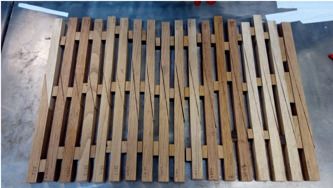
Figure 46 – Samples cut in wright dimension with proper scarf ratio.
