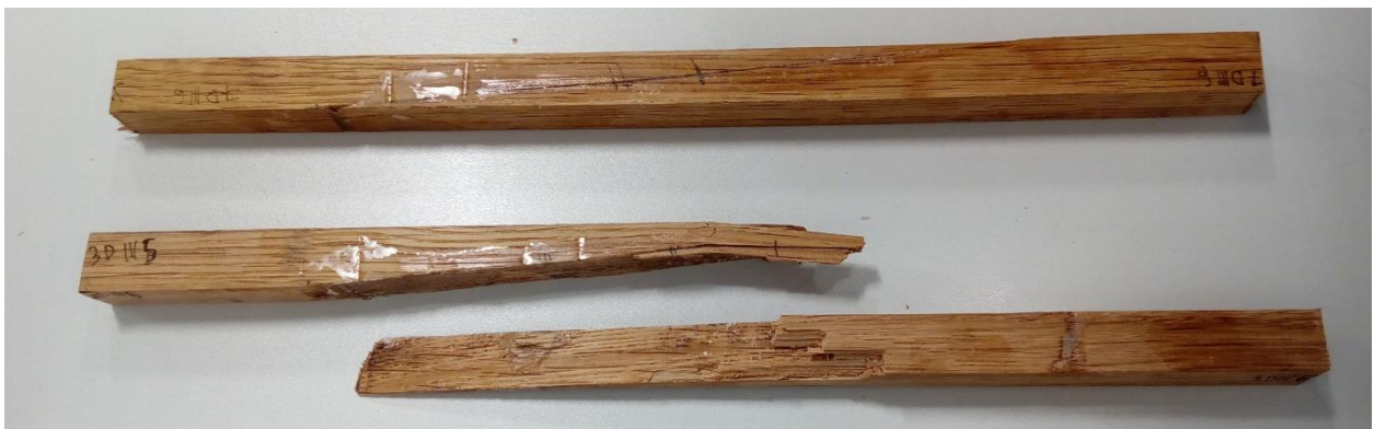
Figure 60 - Samples from 1:12 scarf ratio group – wood failure
