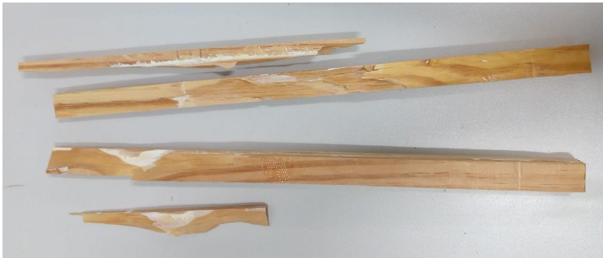
Figure 81– Two samples from control group – wood failure
