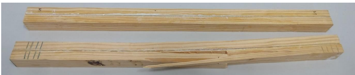
Figure 83– Samples from group with resin film – wood failure
