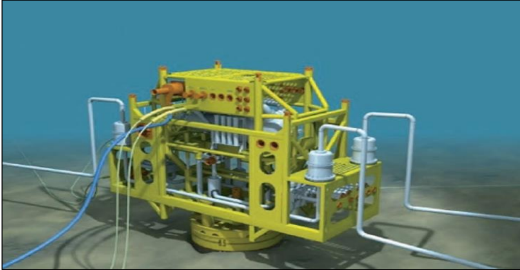
Figure 28 Subsea pressure booster pump
