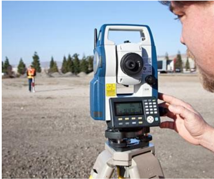
Figure 9 – Measurement Device – X, Y direction – Sokkia Total Station (Product_cx_05.Jpg (375×310) n.d.).
