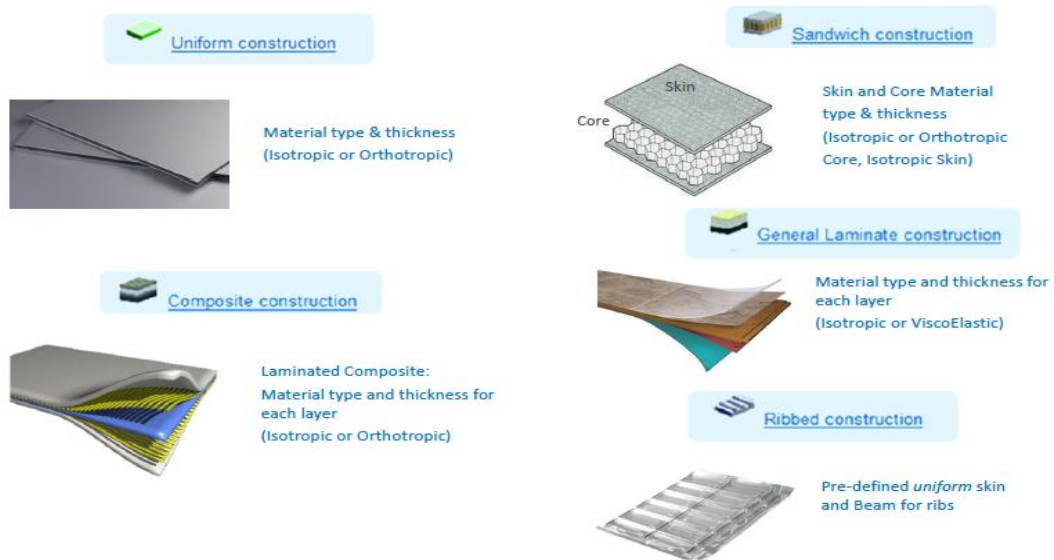
Figure 21: Different forms of plates which can be defined in VA One
