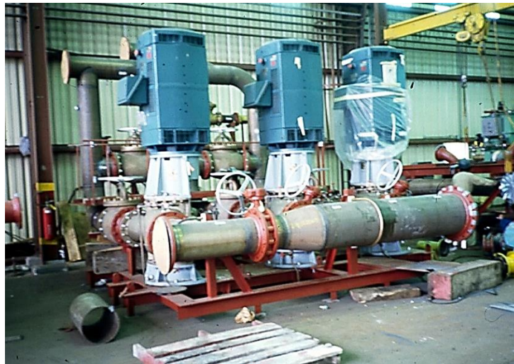
Figure 6. On-unit outfitting package. Pump-set for sea water system. (source: http://i2.wp.com/lou.chirillo.com/wp-content/uploads/2014/06/AVON02b.jpg )
