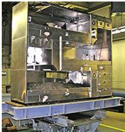
Figure 38. Pre-fabricated galley unit for military ships. (source: http://www.tridentllc.com/military-testing.html )
