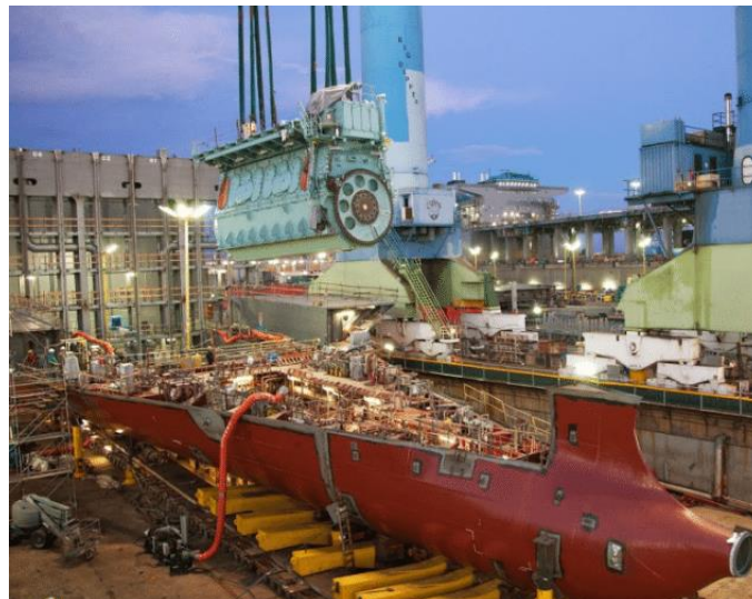
Figure 11. On-block outfitting sample. Diesel Engine Installation. (source: http://gcaptain.com/isla-bella-worlds-first-lng-powered-containership-launched-at-nassco/ )
