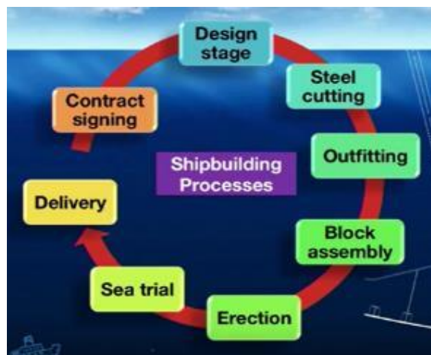
Figure 12. Shipbuilding process cycle including advanced outfitting. (Source: Terengganu Malaysian University – School of Ocean Engineering)
