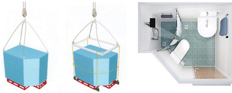
Figure 34. Toilet unit installation configuration (source: http://www.hiseamarine.com )
