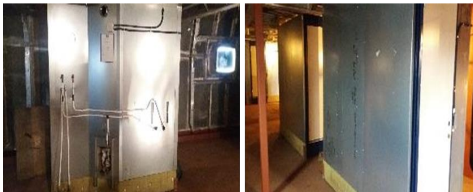
Figure 33. Toilets units introduced in a block before hull assembly (Source: CRIST shipyard)
