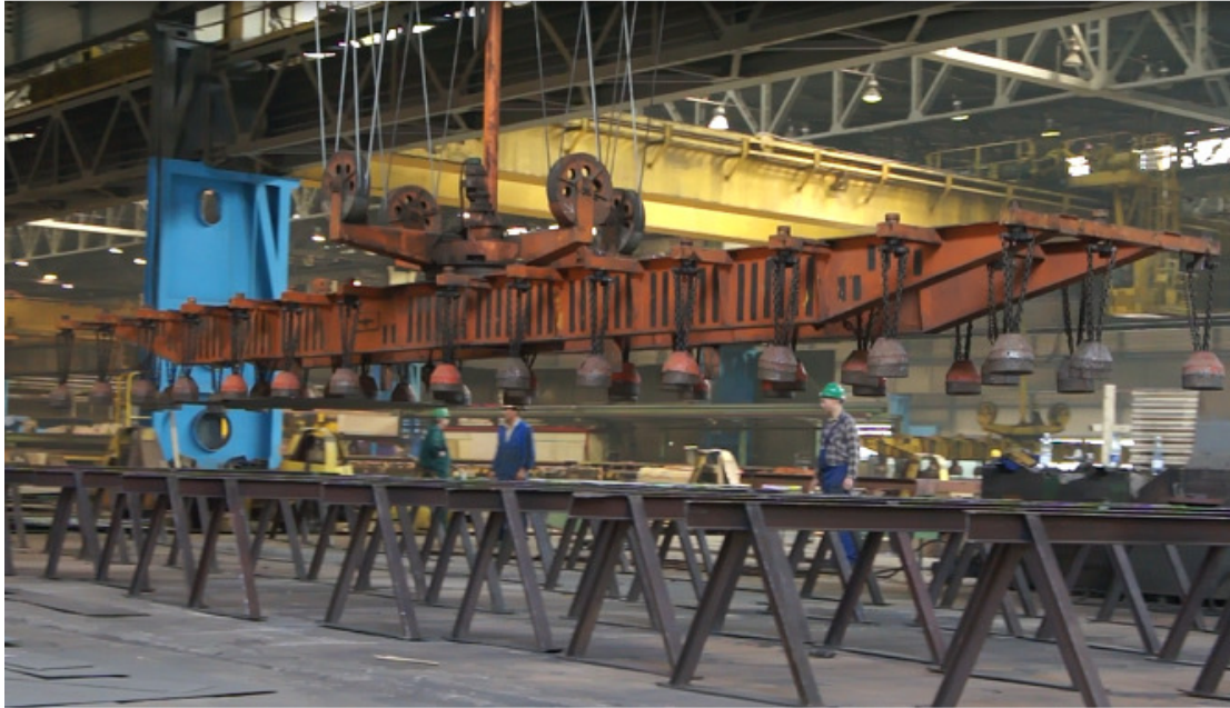
Figure 3.8 - Overhead crane transporting the plates.
