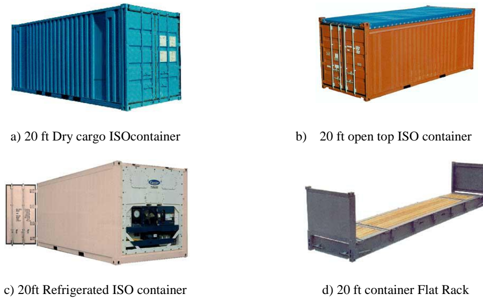
Figure 2.6. Types of containers. Available from http://www.francecontainertrading.fr/htfr/0003.htm [Accessed 23 October 2011].
