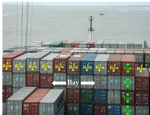
Figure 2.11. Principle of bay-row-tier coordinates; Available from http://www.containerhandbuch.de/chb_e/stra/stra_01_03_03.html [Accessed 10 November 2011].
