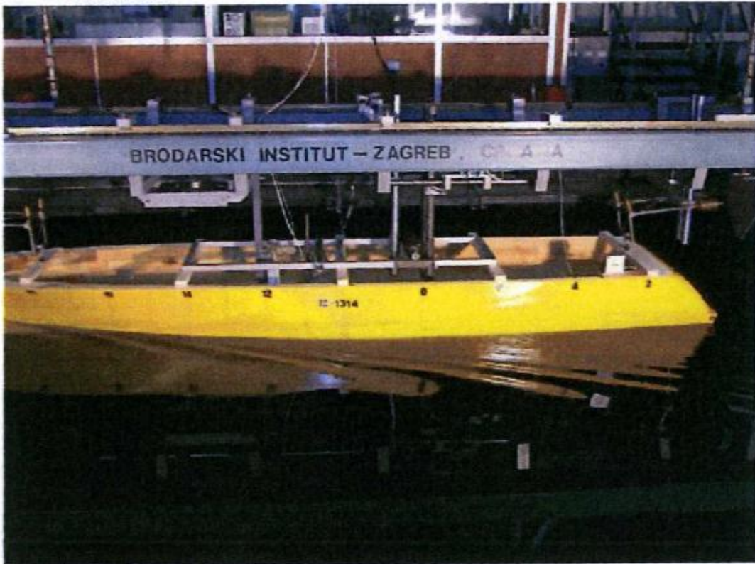
Figure n° 4.8: Model test in towing tank.
