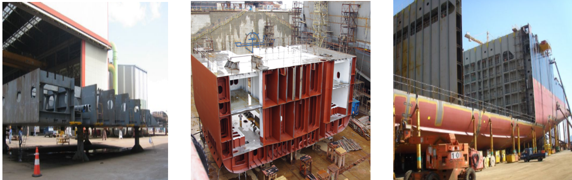
Figure 7. Semi-block, Block and Grand Block Assembly
