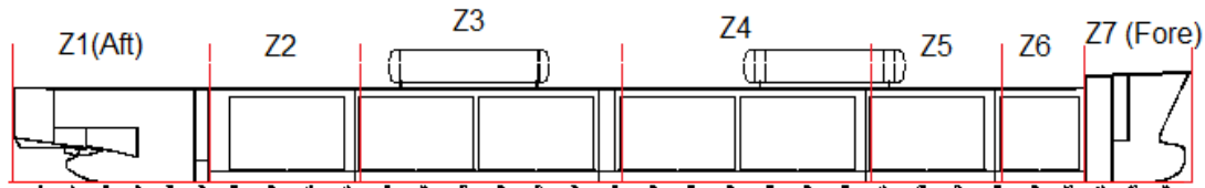
Fig.4.1. Dividing the ship to blocks (Ship Design Group 2007)
