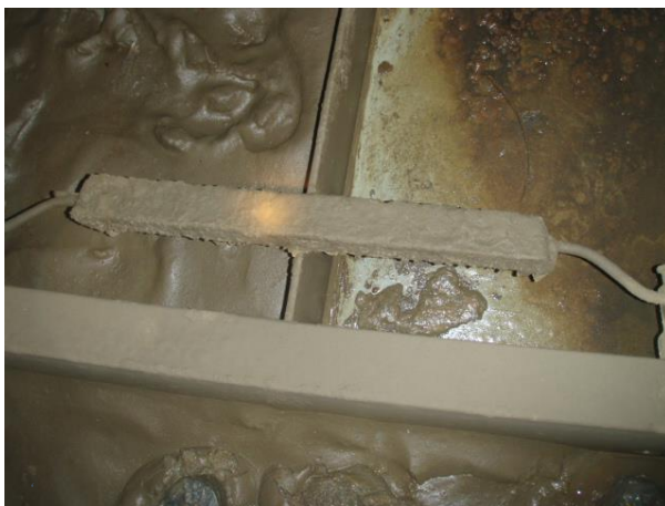
Figure 9 - Sacrificial Anodes inside Ballast Tanks
