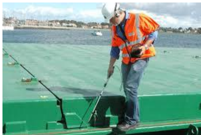
Figure 29 - Ultrasonic Hatch Testing (Source: Damco Survey AB)
