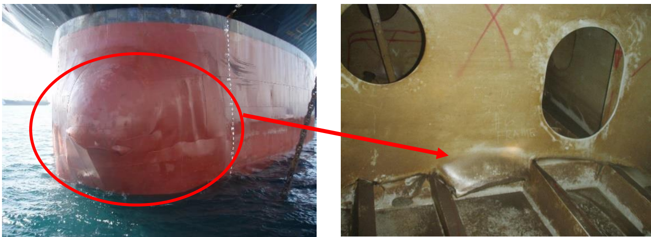
Figure 26 - Bulbous damages due to slamming (Overload)
