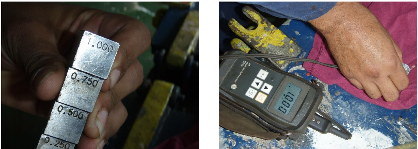
Figure 22 - Calibration block and ultrasonic thickness equipment
