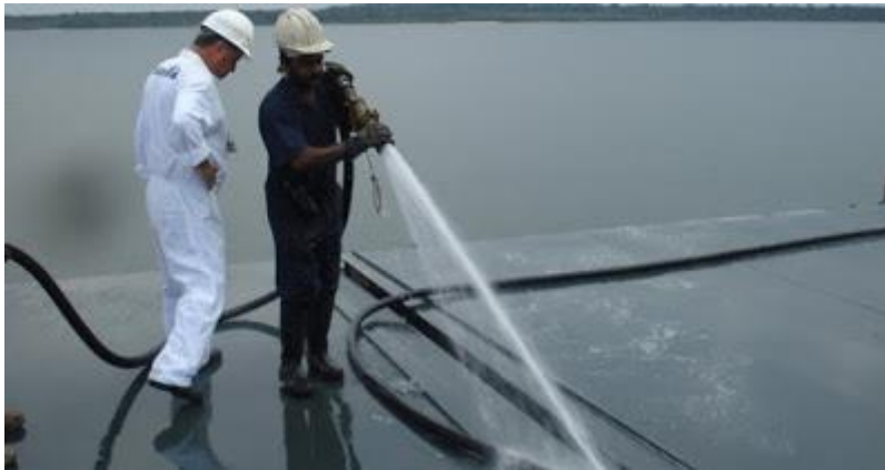
Figure 28 - Hose Test (Source: SS Marine Surveyors)
